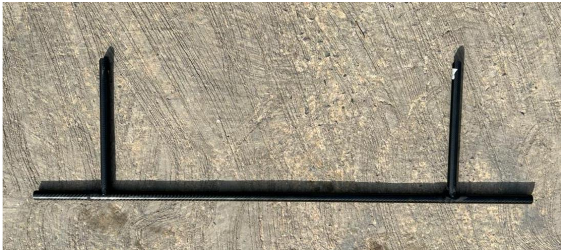
Figure 93 A single skid with epoxy on joints left to dry
