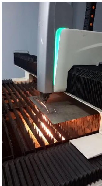
Figure 77. Laser Cutting of mild steel sheet
