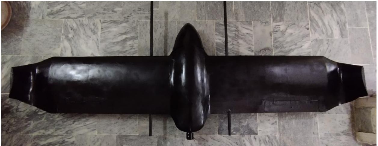
Figure 85. Wing and winglets blended with fuselage
