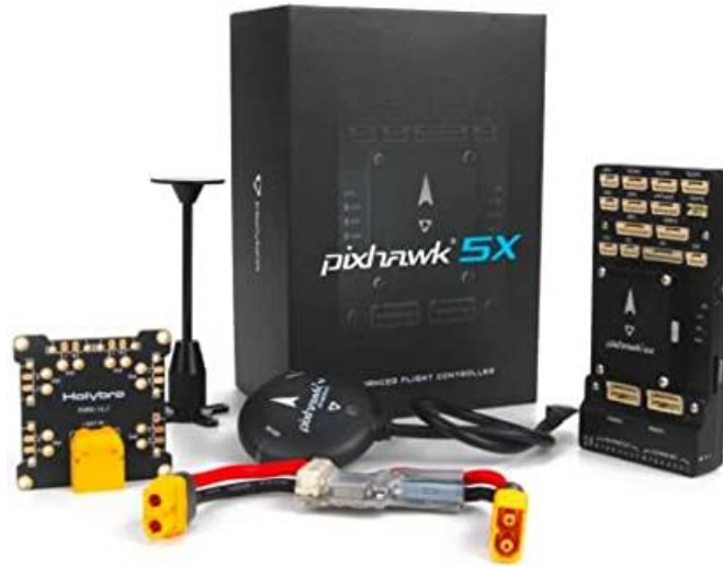
Figure 100 Pixhawk 5X with M8N GPS, Power Distribution Board and other accessories [47]
