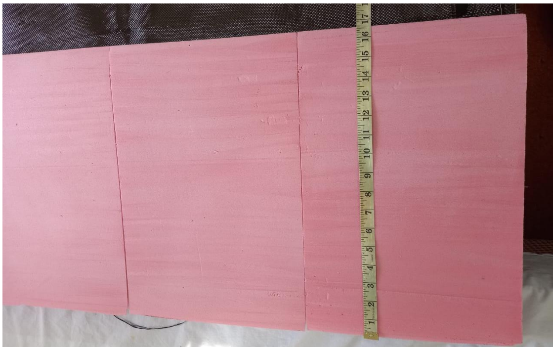
Figure 82. Side view of the foam wing (hot wire cut)
