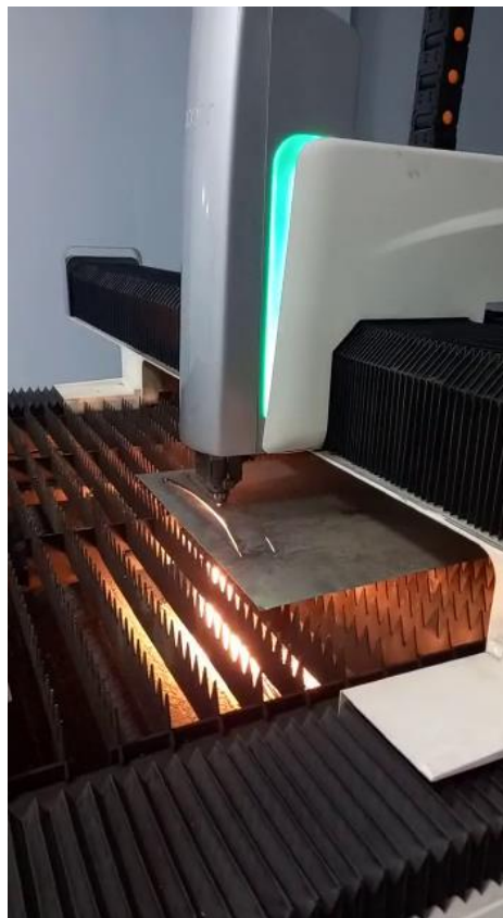
Figure 81. Cutting of airfoil-shaped plates
