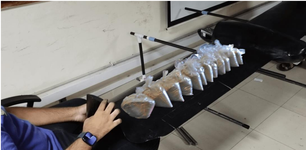
Figure 126 Static Wing Loading Test
