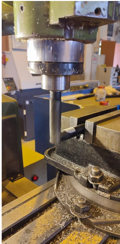
Figure 94 Notching of Booms on a Milling machine
