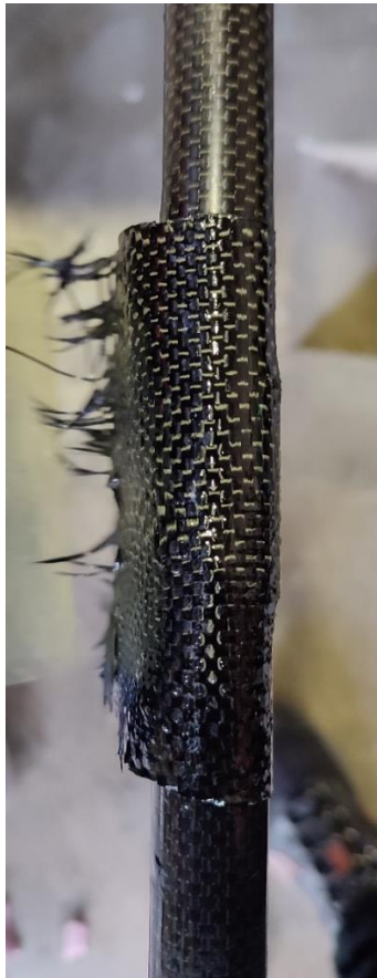
Figure 95 Close-up of CF cloth tape on a boom
