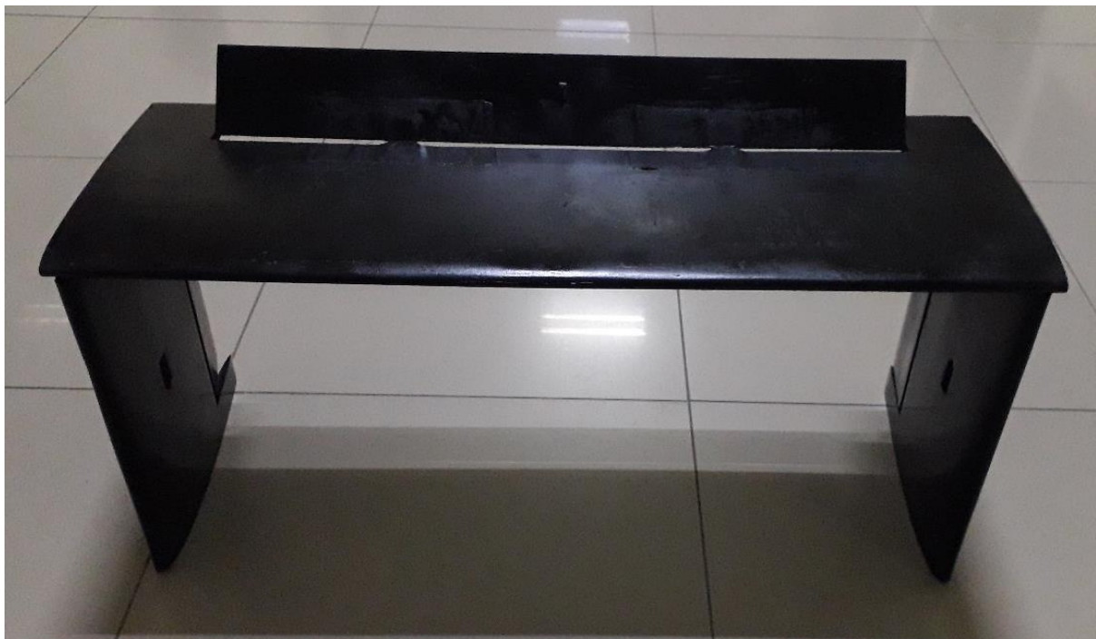
Figure 91 Tail structure (front view with servo slots showing on the insides)
