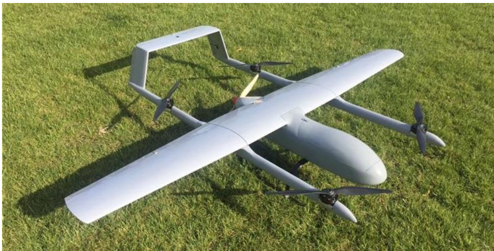
Figure 9 A “4+1” alternating UAV [9]
