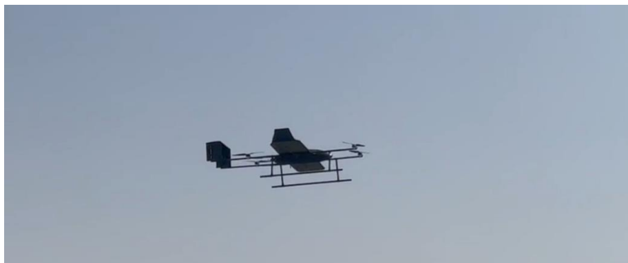
Figure 135 UAV in VTOL Mode 10 m
