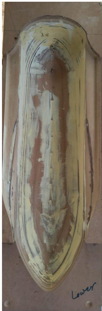
Figure 89 Lower side of Lasani mold for Lower part of Fuselage
