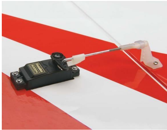
Figure 15 Servo connected to the surface through control rod [16]
