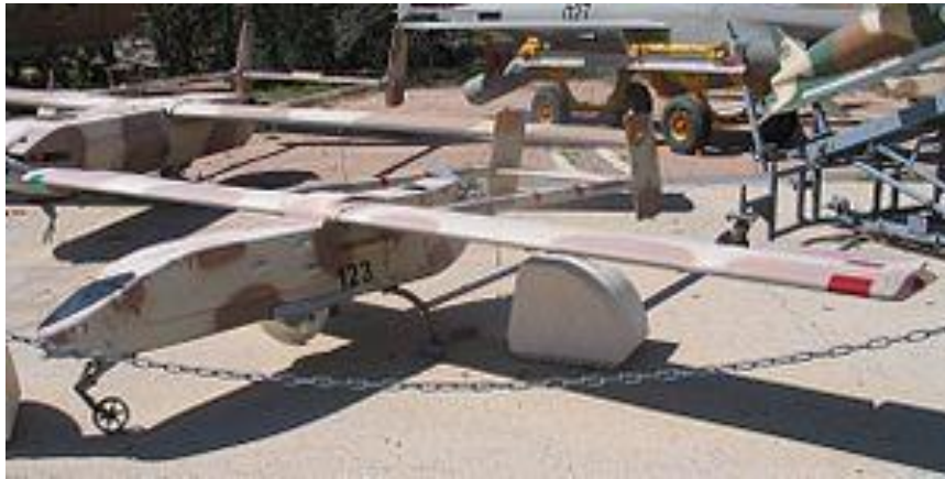
Figure 5 The IAI Scout; a UAV similar in capabilities to its compatriot: the Mastiff [6]
