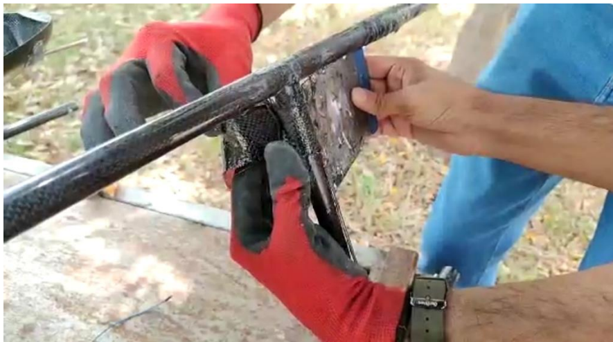
Figure 98 Using scraper to wind the tape tightly
